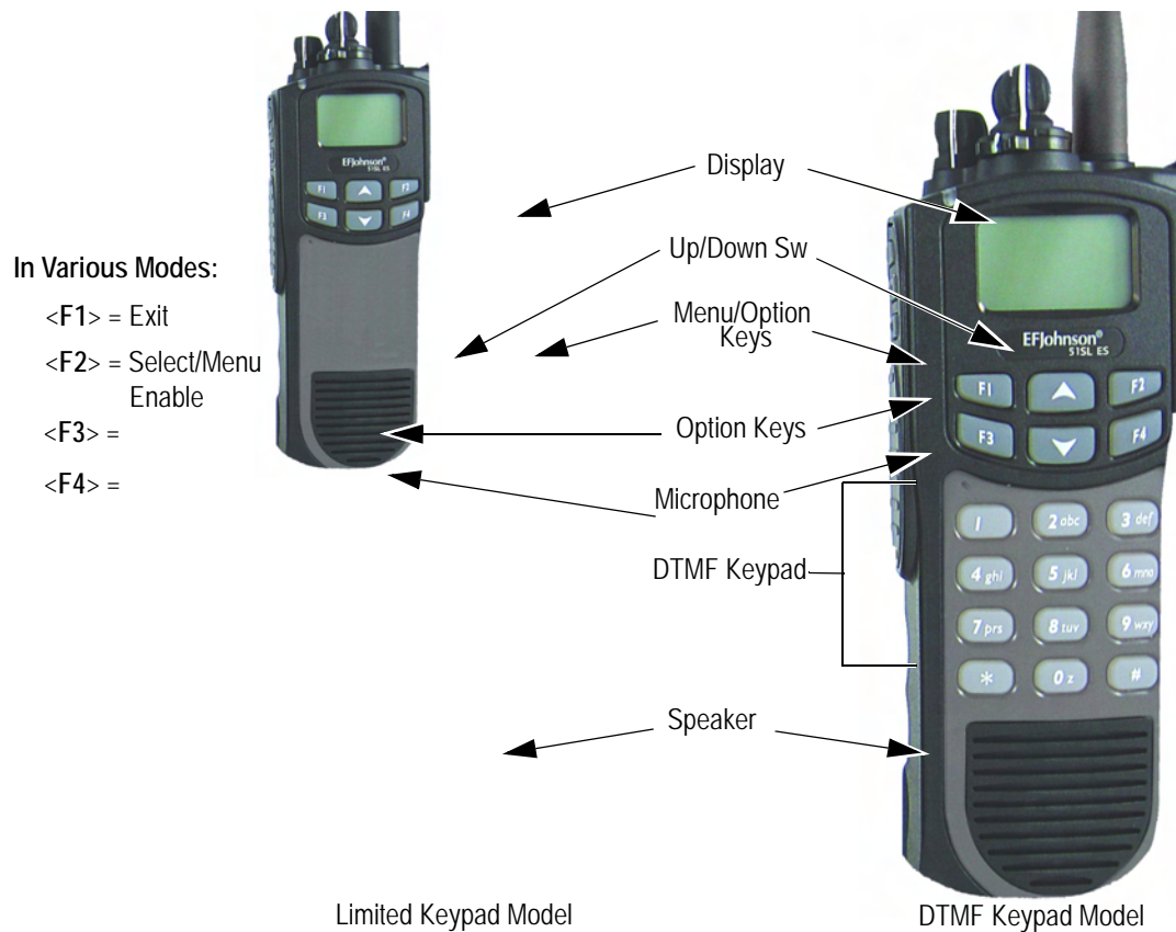
Figure 2.1 Front Panel Controls
