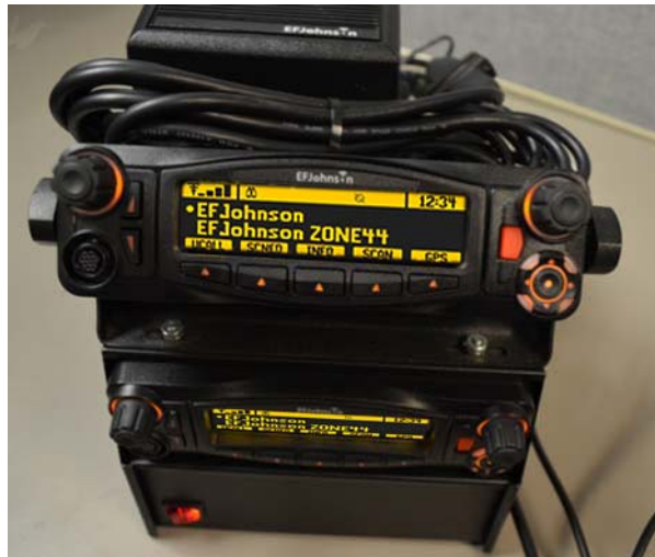
Figure 1.3 Viking Mobile Radio mounted in Base Station
