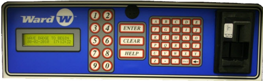
Figure 9.4 Front view of the Front Panel Alphanumeric Keyboard with graphic LCD and magnetic card reader.
