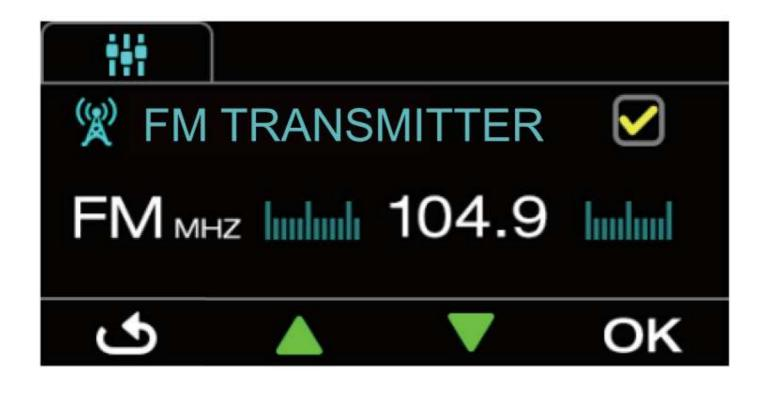
NOTE Please be informed that the poor reception may occur when the frequency signal of the radio station is stronger than the FM transmitter.
