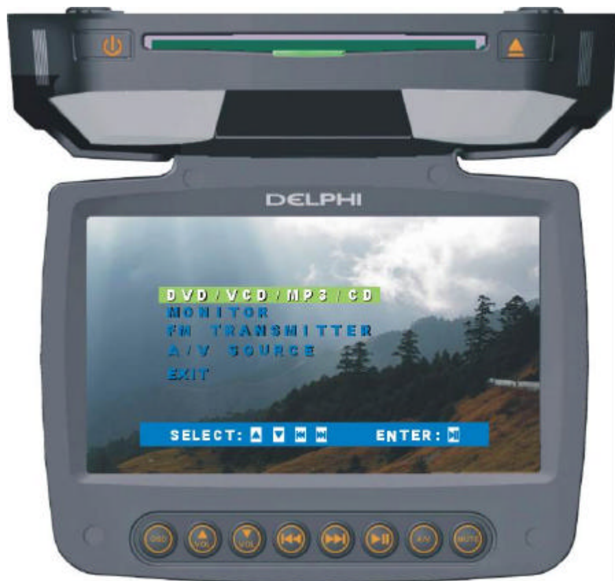
Figure: Main section of OSD
