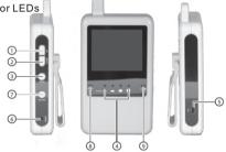
NOTE: ON/OFF: Press and hold button for 3 to 5 seconds. ESC: Press and quickly release button.
