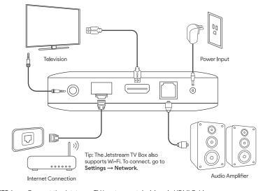
Please refer to the diagram below for connecting your Jetstream TV Box to power, network and other devices. (Note: Before getting started, please shut down all equipment to be connected.)
