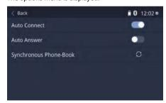
**Auto Connect** – If "Auto Connect" is activated, the device automatically connects with known Bluetooth® devices as soon as they are in range.
