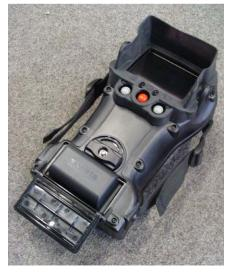
• Turn on the unit using the middle RED button on the rear. A RED light will be illuminated in the position shown. A long (3 second) press is required to switch the camera off.
