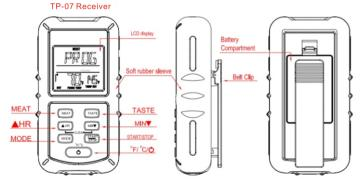
LCD (Liquid Crystal Display) – Displays all icons, temperature and timer. The back light will flash Blue once the temperature increases  $10^{\circ}F$ , will change to Green when the temperature is within  $15^{\circ}F$  of the set temperature and will turn Red when it reaches the set temperature. See LCD diagram for detailed information.
