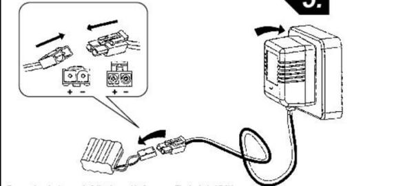
Ensure that the battery is fully charged before use. The included 7.2V Vehicle Battery Pack is NOT charged prior to shipment, please charge for 8 hours (first two full charges) out of the box.
