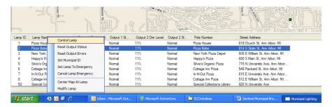
Select control lamp to display the control window for the selected lamp. The lamp can be controlled as described previously.
