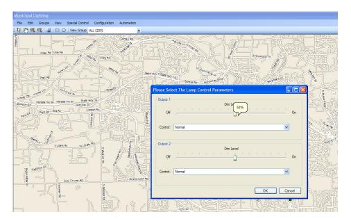
Use the mouse to move the sliders to control the **Output1** (white for San Jose) and **Output2** (Yellow for San Jose) light amplitude to the required level. Click OK to send the signal.
