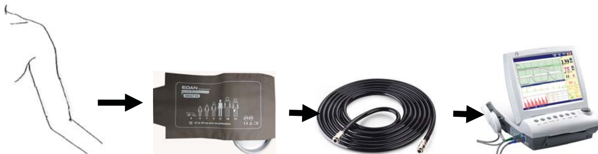
Figure 9-5 Connection for NIBP measurement
