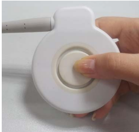
Figure 7-6 Testing a TOCO Transducer
