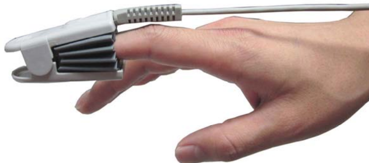
Figure 9-3 Placement of the Finger for SpO 2 Measuring
