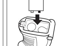
1) Open or close the cover with 2) Insert 1 9V (6LR61) Alkaline
