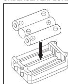
I) Open or close the cover with a Philips screwdriver. 2) Insert 3 size "AA" (LR6) 1.5 V batteries.
