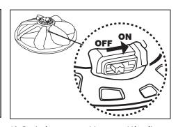
1) With your Vectron Ultralite on 2) S witch on your Vectron Ultralite. the launch platform, unplug the charging cord.
