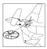
A) Battery Compartment Unit: uses 6 "D" size batteries. Ensure both the AIRIDER and the Radio Controller is switched to the OFF position. Insert the battery compartment unit power plug into the DC socket of the AIRIDER.
