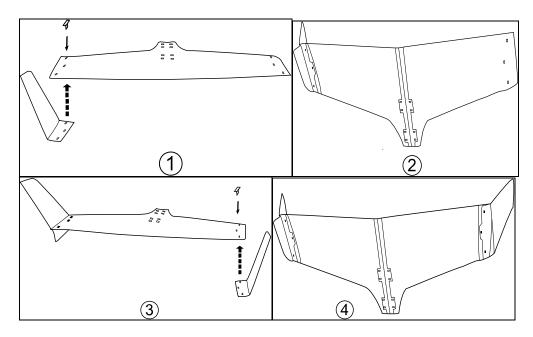
Secure your AIRIDER to the main wings by inserting the fuselage fasteners.
