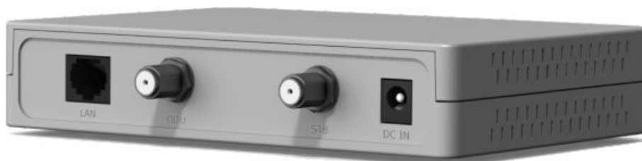
Fig.23. Indoor Unit's rear panel.
