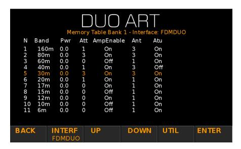
Using the "UP" and "DOWN" button it is possible to go through the table and modify it.
