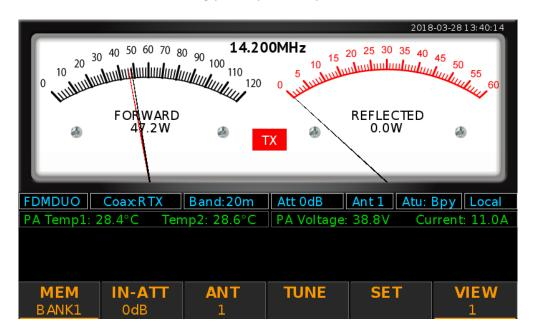
The configurations are saved in memory banks, and it's possible to switch between them pressing the "MEM" button. The banks can be added or deleted until a maximum of 20 banks. The two underlined button (MEM and VIEW) have a second function if pressed longer.
