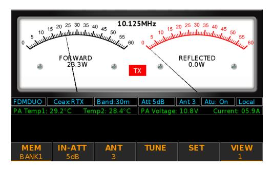
The configurations are saved in memory banks, and it's possible to switch between them pressing the "MEM" button. The banks can be added or deleted until a maximum of 20 banks. The two underlined button (MEM and VIEW) have a second function if pressed longer.
