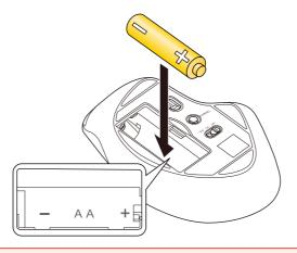
Ensure that the battery is inserted with the positive (+) and negative (-) terminals oriented correctly.
