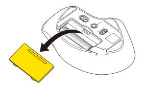
2) Remove the battery insulating tab.
