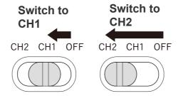
When paired with only one device on either "CH1" or "CH2", the existing connection will be lost when you switch to the unpaired channel.
