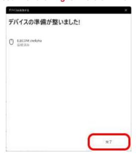
9) Pairing is complete when this product is added to "Bluetooth & devices" and the status is "Connected".
