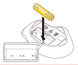
Ensure that the battery is inserted with the positive (+) and negative (-) terminals oriented correctly.
