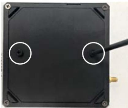
3. Hold the case towards the VESA bracket and insert the screws into the holes.
