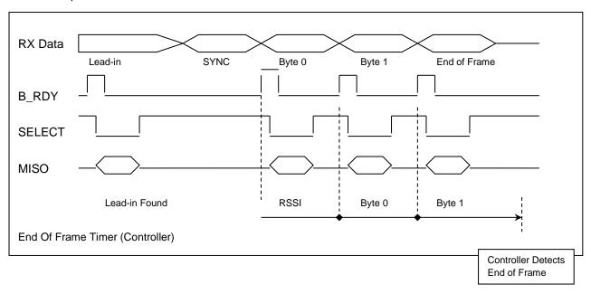
If the radio loses lead-in lock before the sync word is received, then an RSSI value of 0xFE is transferred to indicate no more data to follow. The Lead-in Found code is 0xFF.
