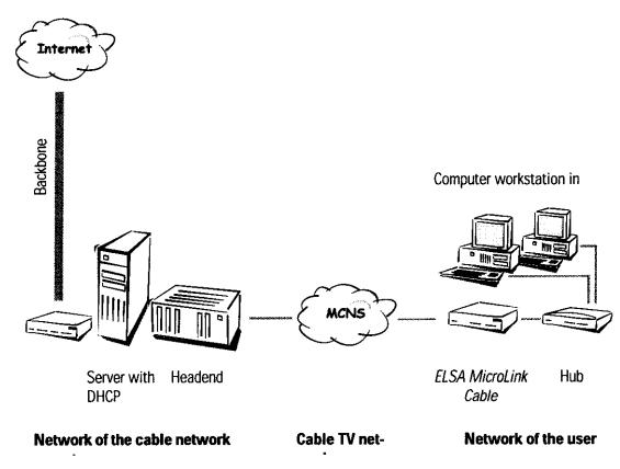
This connection to the backbone is of little relevance to the user. However, the greater the of the network operator's backbone line, the quicker the users receive information from the Internet.
