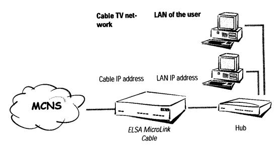
The cable modem is therefore assigned a cable IP address and a LAN IP address, each with its own appropriate network mask. Use the 'Masquerade' option to inform the cable modem which of the two addresses to use when transferring the packets.
