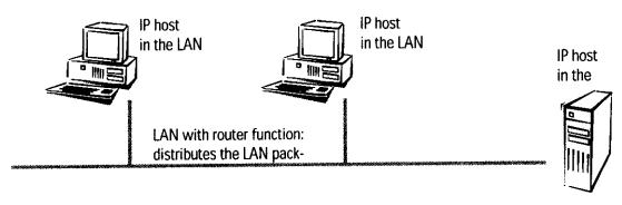
To a router in the LAN, a host in its own LAN seems to be located behind another router. So the task for the router is very simple: all it has to know for operating in the IP network are the IP addresses
