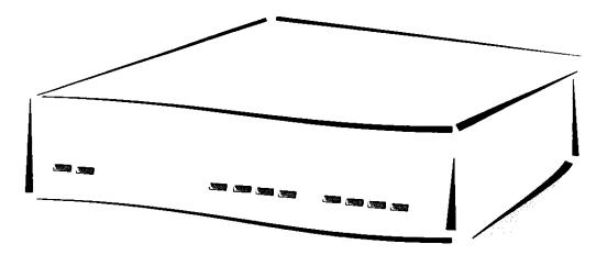
This LED flashes once when the power supply is switched on. After the self-test, either an error is output by a flashing light code or the device starts and the LED remains lit.
