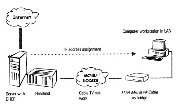
In this example, only one computer is connected to the Internet via the ELSA MicroLink Cable. In principle however, several computers can be connected to the ELSA MicroLink Cable, using a hub for example.
