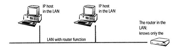
In contrast, the host is confronted with a more difficult task than the router. In case of an interface with a point-to-point cable, the host knows that all packets that it sends through the interface automatically arrive at its router, for example. In case of the point-to-multipoint connection to the LAN, it has to distinguish two cases, however.
