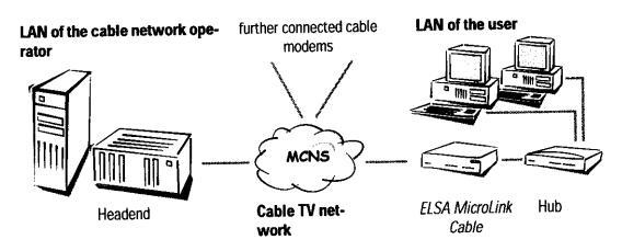
In the bridge operating mode, the *ELSA MicroLink Cable* transfers all data to computers without locally assigned MAC addresses, between the local network or another local area network (LAN) or a workstation on one side and the cable network on the other side.
