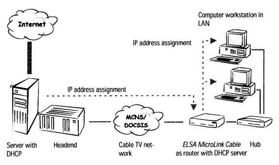
In this example, several computers are connected to the ELSA MicroLink Cable, and thus to the Internet, using a hub. In principle however, a single computer can also be connected directly to the ELSA MicroLink Cable.
