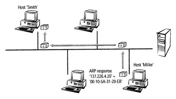
Then it can finally turn to its original task: sending the IP packet to host 'Miller'. It now finds the entry "IP address 137.226.4.20 corresponding to MAC address '00-10-5A-31-20-EB'" in the ARP table and tells his LAN interface: "Send this IP packet to the computer with the MAC address '00-10-5A-31-20-EB'".
