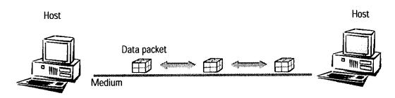
Access to the Internet is also established through point-to-point connections. Even though the data packets are sent from the host at the Internet user to the host at the Internet provider (server) via several routers, every data packet still has its own specific destination. Furthermore, the routers will only forward the data packets to one recipient. That's why we also call this connection unambiguous.
