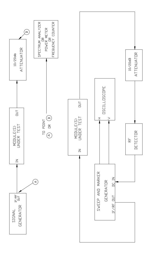
TEST EQUIPMENT SETUPS FOR MEASURING THE GAIN OR LOSS OF THE MODULES
