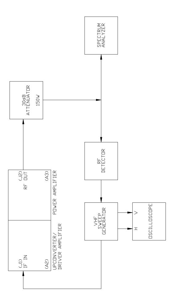
ALIGNMENT OF RF AMPLIFIER CHAIN FIGURE 3-4
