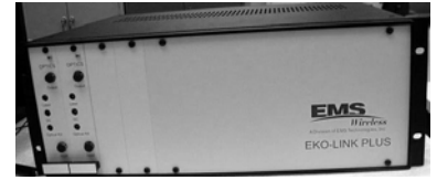
Typical EkoLink Plus Hub front panel shown with two RF/Optical Transceivers Installed
