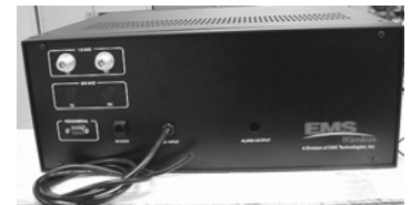
Typical EkoLink Plus Hub Rear Panel with 1900 MHz only
