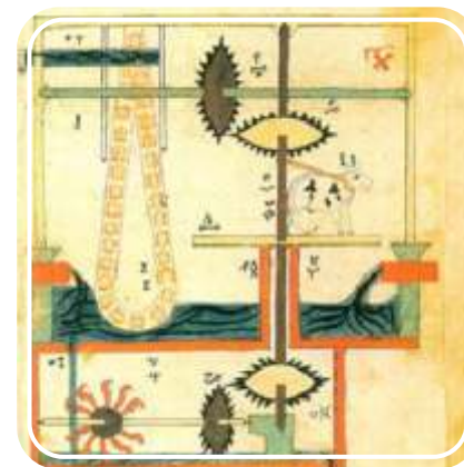
Al-Jazari's drawing of a hydropowered chain pump
