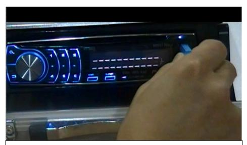
Turn audio on. Plug Multishare 1.0 into audio USB port. Ensure that the LED light blinks.
