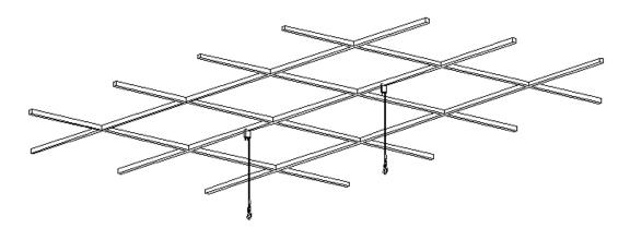
3.2 Place the provided V type hook over the hook of each rope hanger. Ensure both end of rope hanger are secure.
