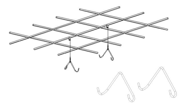
3.3 Hold the fixture body by hands, and hang the fixture body by placing one V type hook over each hole on both side of the fixture, adjust the rope hanger to level light.
