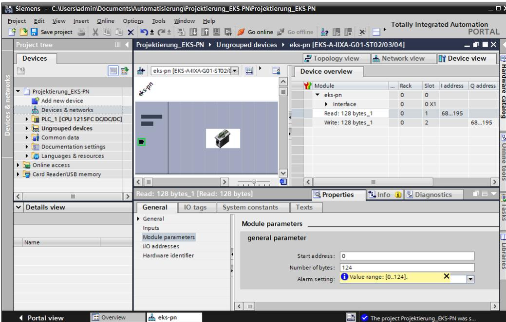
8. In the module *EKS write*, set the required alarm mode.
