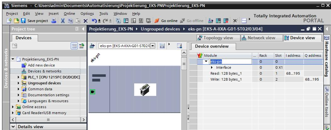
10. If required, you can change the input address area in the control system for the module *EKS read*.
