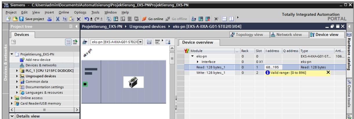
11. If required, you can change the output address area in the control system for the module *EKS write*.
