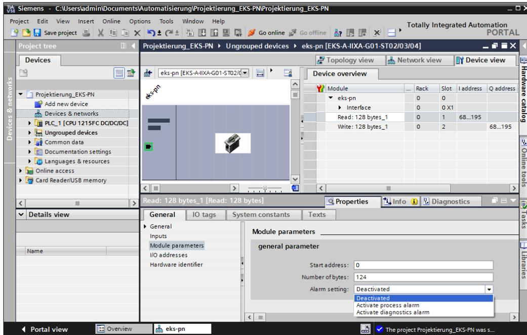
6. In the module *EKS read*, set the start address from which the data on the Electronic-Key are to be read.
