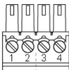
Plug-in connection terminal, 2 x 2-pin, with screw terminal
