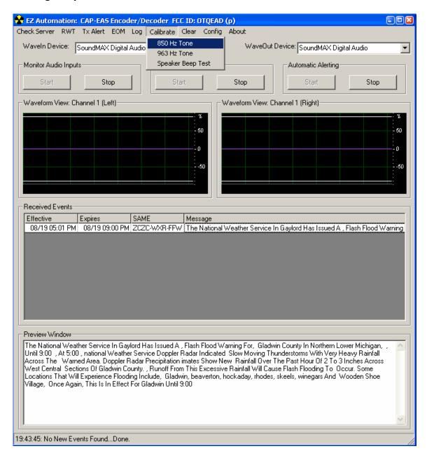
You may test and set the audio output levels by clicking on menu then on **Calibrate** and then either **853Hz** or **960 Hz** tone button. This will allow the adjustment of audio levels in the broadcast facility produce at least 40% modulation as required by FCC rules at the time of writing.
