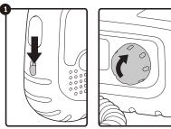
Slide the Walkie Talkie Switch down to turn the Walkies ON. Rotate the Base Station Knob clockwise to turn Base Station ON. The knob is also used to control the volume of the Base Station.
