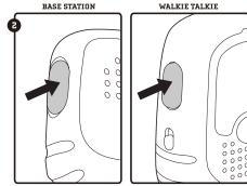
Press and hold the Push To Talk Button to transmit sounds. Release the Push To Talk Button to receive signals. A squeaking noise will be heard if the base station and Walkie Talkies are too close.
