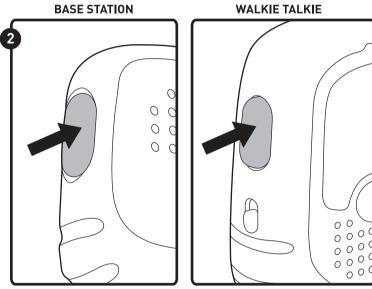
Press and hold the Push To Talk Button to transmit sounds. Release the Push To Talk Button to receive signals. A squeaking noise will be heard if the base station and Walkie Talkies are too close.
