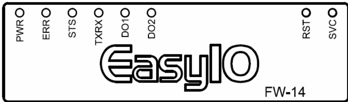
Image shows the Status indicator, Error indicator and individual Digital Output indicator Button and LED indications. Image shown is an EasyIO FW-14.
