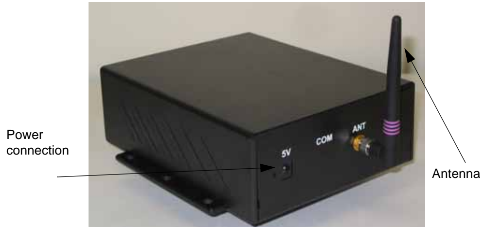
Figure 6.6 Indoor Gateway - Power Connection
