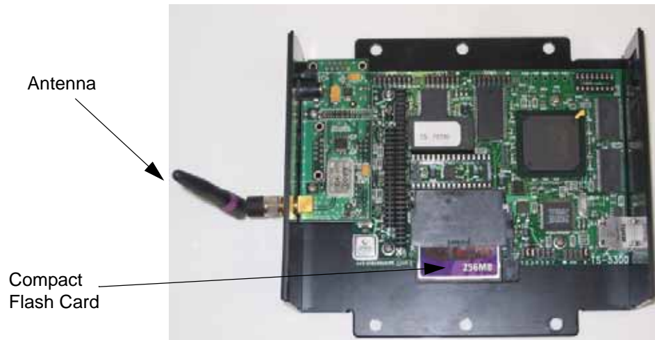
Figure 6.7 Indoor Gateway - Cover Removed
