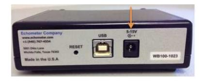
3. Connect the supplied USB cable between the **Echometer Computer** and the WB100 USB port.
