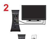
Connect the other end of the cable to the appropriate input of your TV or monitor. Confirm that both your TV and the Wireless Joey receiver are connected to a power outlet. **Note:** In most cases, connecting the HDMI cable provides plug-and-play control of the TV's display resolution and other settings. However, your TV may require selecting a different format to display from the Wireless Joey receiver during setup.
