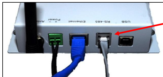
Figure 10 – Location of serial connection in back of Gateway
