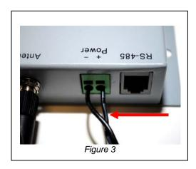
Note: Please ensure proper polarity before plugging the power supply into an electrical outlet.
