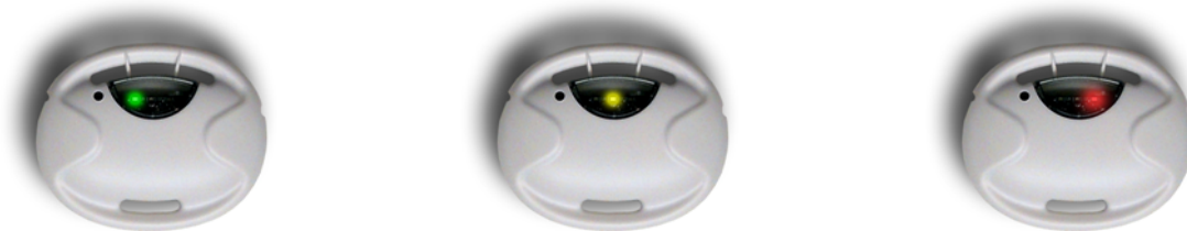
Figure 2. HCWs Badge LEDs: Green (Sanitary State), Yellow (Cautionary State) and Red (Warning State)
