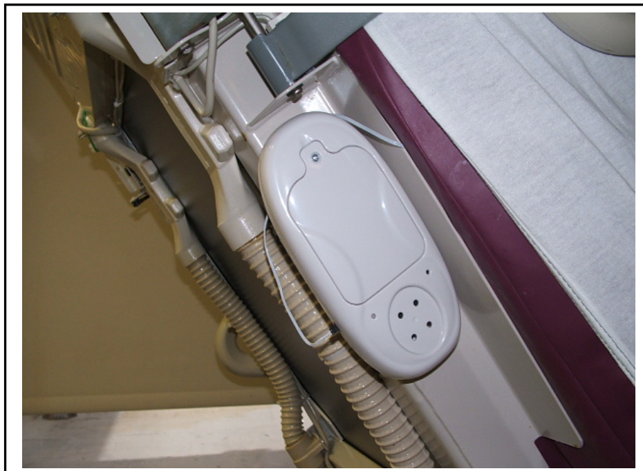
Figure 6. Bed Beacon Mounted on Patient Bed
