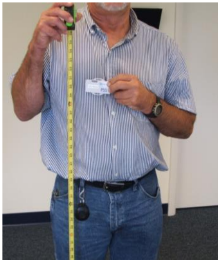
Figure 9. Test Badge Height Is 50 Inches From the floor
