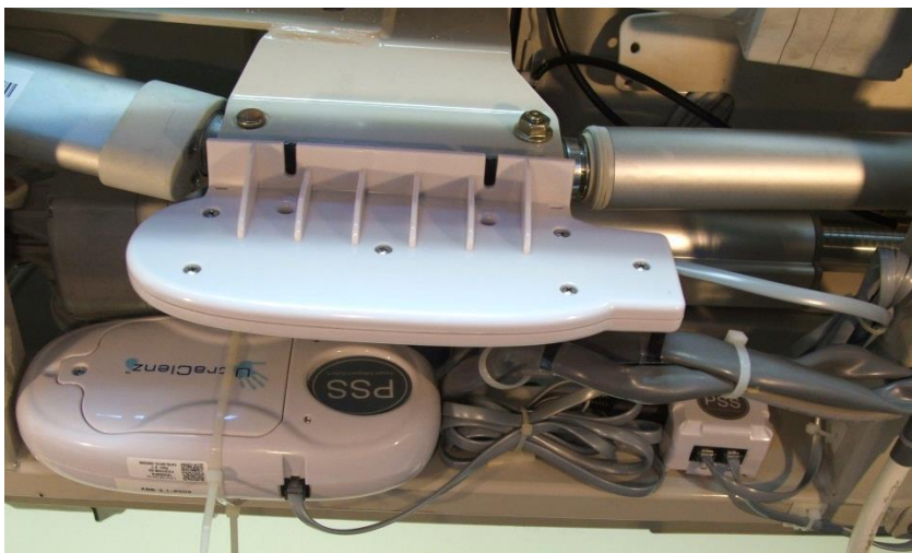
Figure 3. Bed Beacon Mounted on Patient Bed Model Hill-Rom Versa Care P3200
