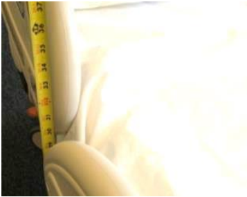
Figure 8. Adjust Bed Mattress Height to 30 Inches
