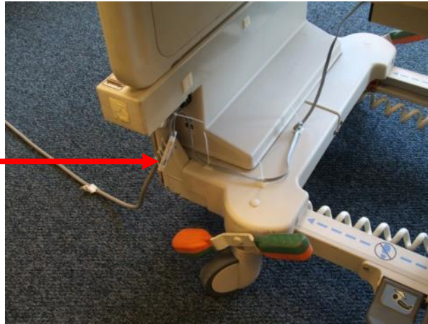
Figure 6. AC Line Power Sensor Attached to Power Cord
