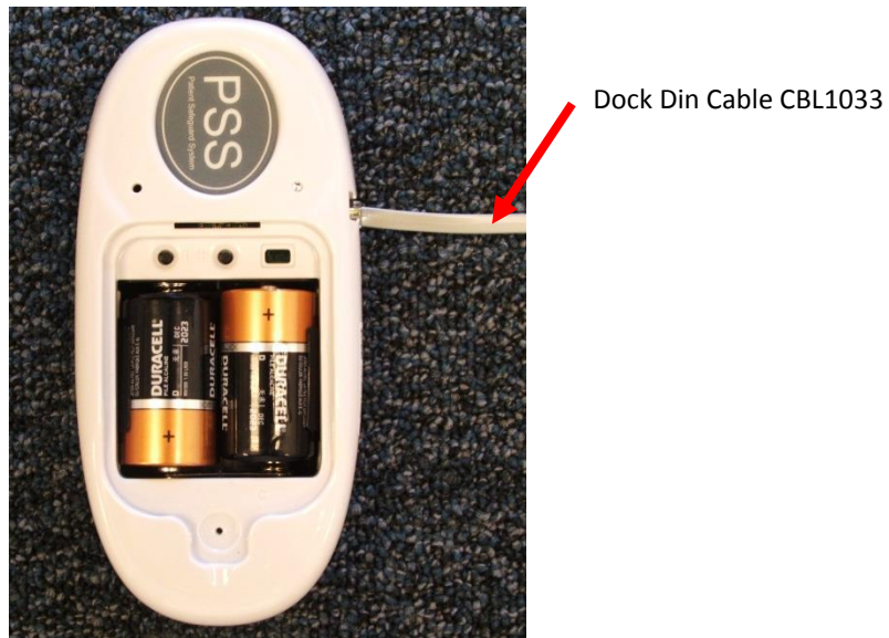
Figure 4. Connecting the Bed Beacon to the Dock
