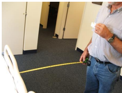
Figure 10. Test Badge Activation Distance from Bed's Handrail Center is 24"
