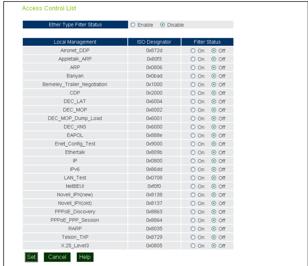
Figure 31: Ethernet Type Filter
