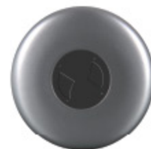
Fig.1: Firmly hold the remote whilst pushing down the black cover underneath the remote and twist cover to the left.
