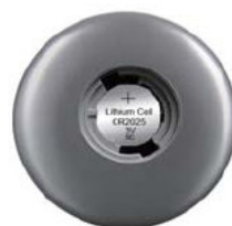
Fig.2: Battery must be inserted at a slight downward angle towards metal retaining clip. Battery must sit flush in the housing. The positive symbol (+) must be facing up as in the photo.
