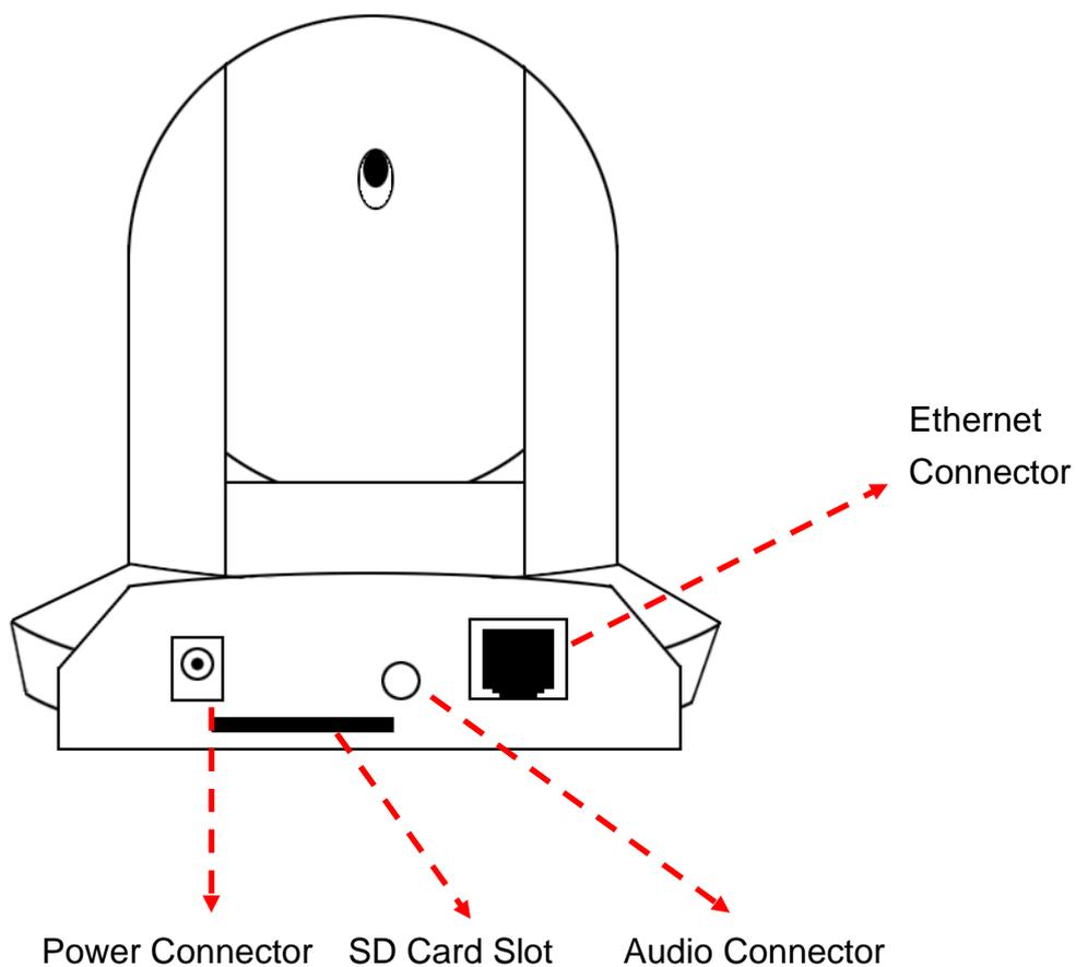
Power Connector: Connects to 12V DC power adapter
