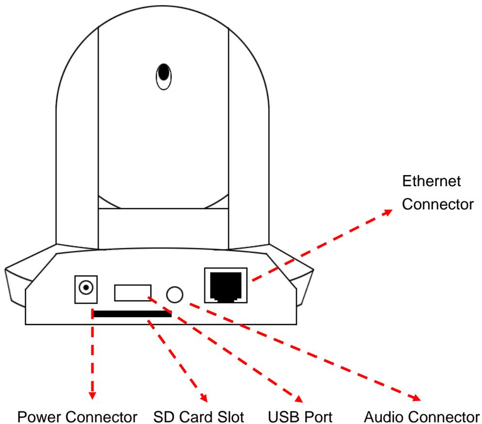
Power Connector: Connects to 12V DC power adapter
