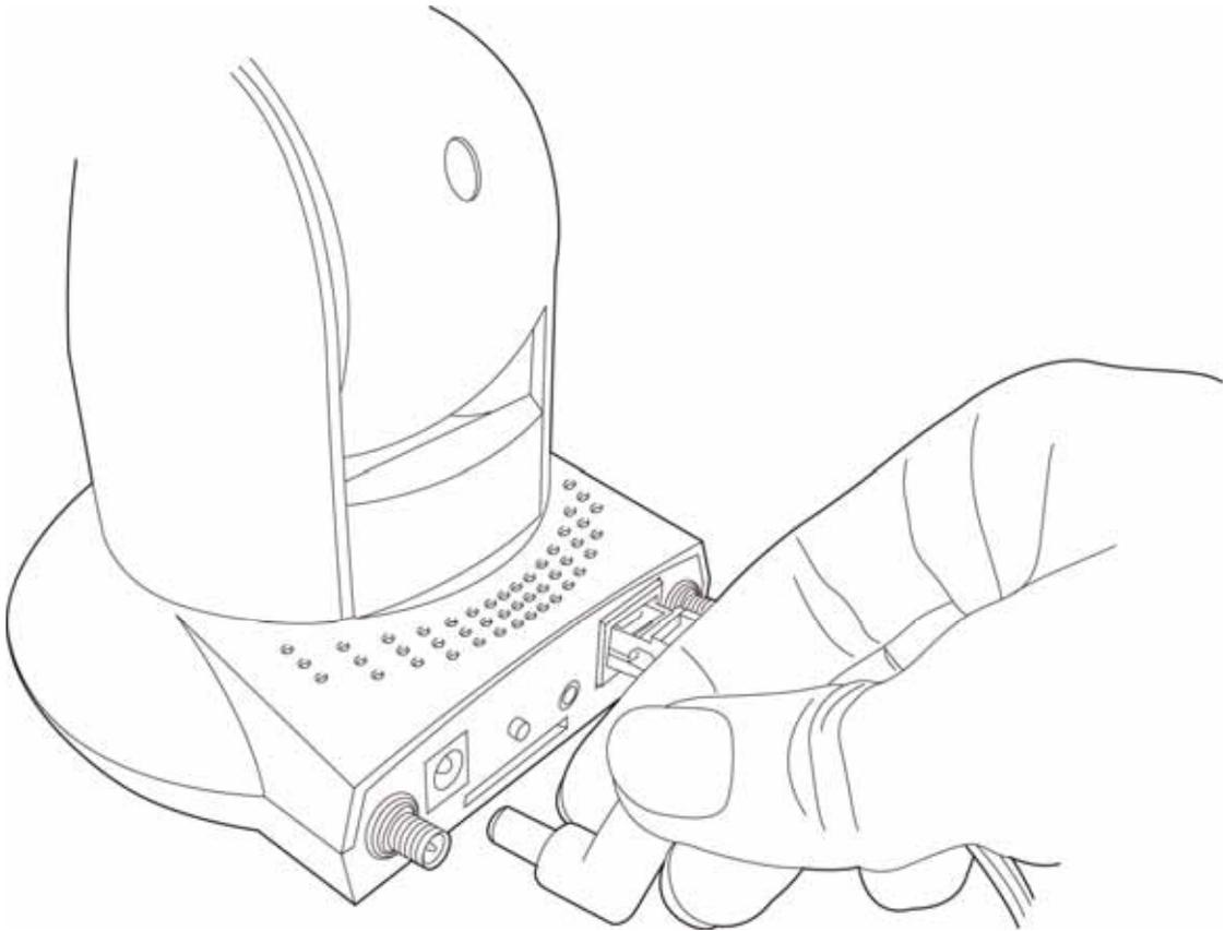
4. Connect two antennas to the antenna bases, which is located at the back of this IP camera.
