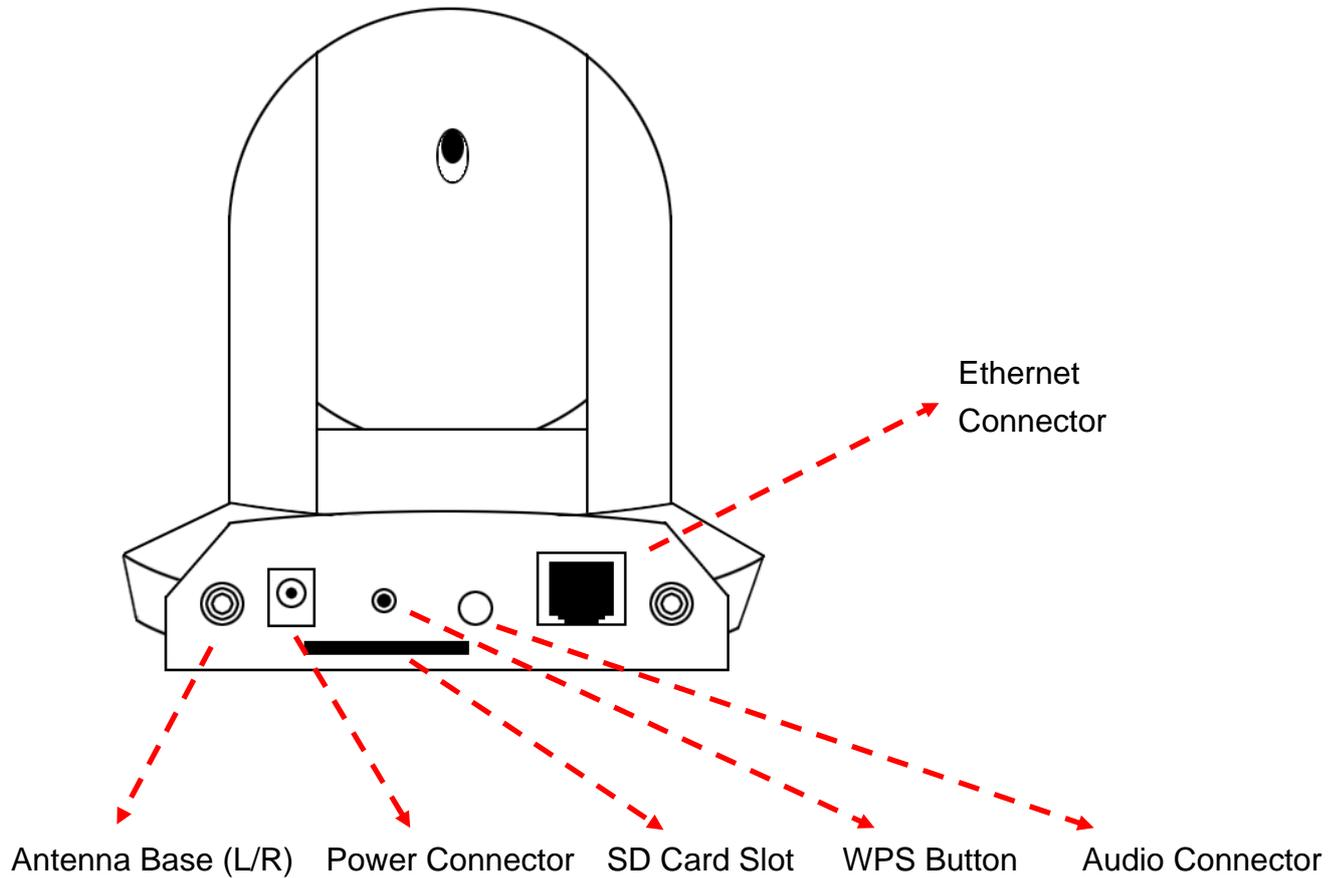
Antenna Base: Connects to supplied antenna
