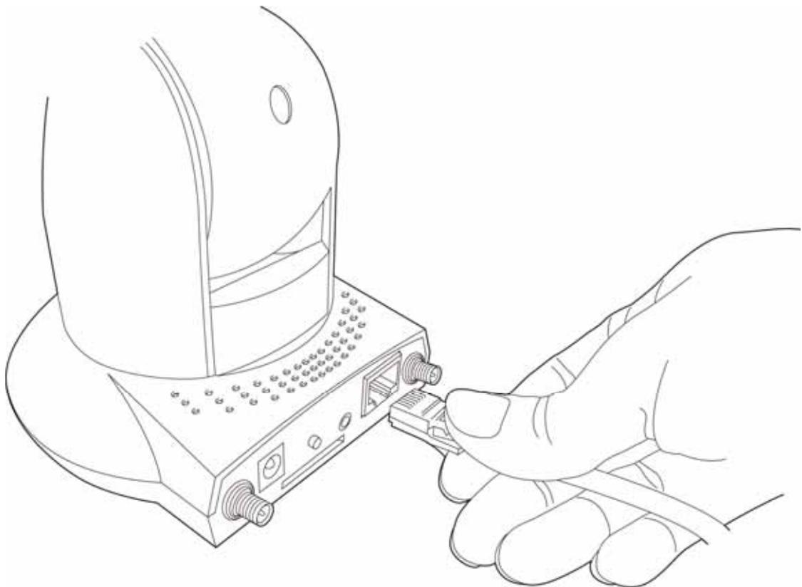
3. Plug the power adapter to wall socket, and connect the power connector to the power jack located at the bottom of the IP camera.
