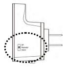
Insert this device into power outlet on the wall, and switch wireless repeater's power switch to '**ON**' (1). You should see '*Power*' LED light up in few seconds (2). If not, please check if the power outlet you're using is working.
