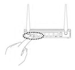
NOTE: this WPS button position on access point is for example, different device may have different WPS button position.
