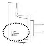
Insert this device into power outlet on the wall, and switch wireless repeater's power switch to '**ON**' (1). You should see '*Power*' LED light up in few seconds (2). If not, please check if the power outlet you're using is working.
