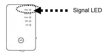
(4) Please move repeater to the place you wish to use (a better place will be the center of your house) and insert this repeater into power outlet on the wall, the wireless connection will be established automatically. You can check '*Signal*' LED status to understand signal reception level. Steady light: Excellent, Flash: Good, Fast flash: poor.
