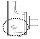
Insert this device into power outlet on the wall, and switch wireless repeater's power switch to ' $\mathbf{ON}$ '(1). You should see '*Power*' LED light up in few seconds (2). If not, please check if the power outlet you're using is working.
