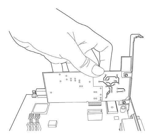
Tip: It's recommended to touch some metal material before installing the network card, or the static on your body may damage the components on network card and computer.
