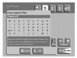
Enter a name for the playlist using the alphanumeric keys on your VIA!dj remote control or using the grid.
