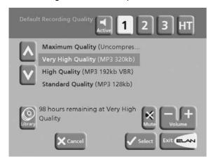
For each quality setting the screen shows the number of hours of recording time available at that setting.
